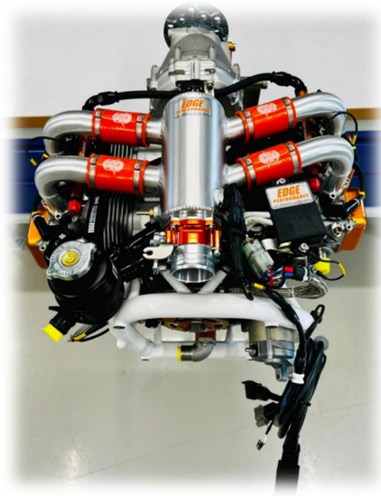
13 Picture showing a typical installation of the EFI system onto a Rotax 912ULS engine.
