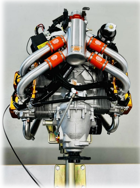
14 Alternative hydraulic governor intake design when installed on engines with hydraulic propeller governor, DUC, Eprops hydraulic actuator etc.
